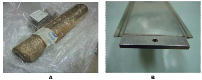
Figure 45. (A) Ag-In-Cd ingot for Control Plates; (B) Laser welded stainless steel envelope to house Ag-In-Cd and for use as IEA-R1 control element.
