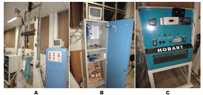
Figure 52. (A) VAR furnace; (B) command "box"; (C) retrofitted power source.
