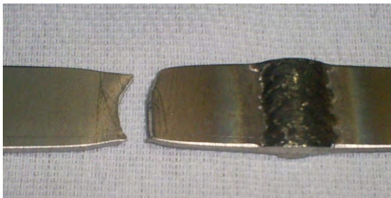
Figure 39. Specimen with a reworked weld joint following a tensile test.
