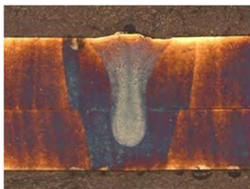
Figure 40. Macroscopic image of the fiber laser welded joint.
