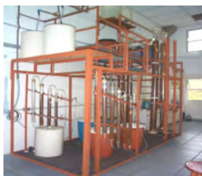
Figure 26. Rare Earths pilot plant at IPEN-CNEN-SP.
