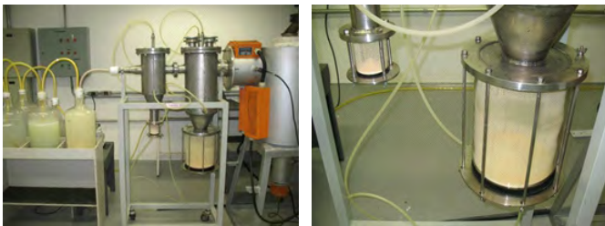
Figure 47. Chlorination process of zirconium oxide.
